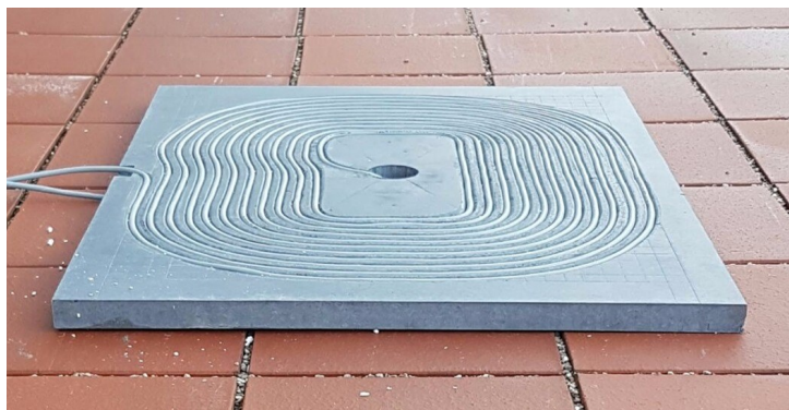
Fig 3. MAGMENT concrete plate with embedded coil
