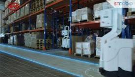
An unmanned forklift successfully completing obstacle avoidance and path selection
