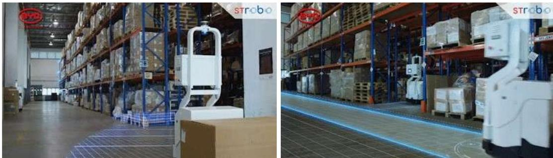
*An unmanned forklift successfully completing obstacle avoidance and path selection*
